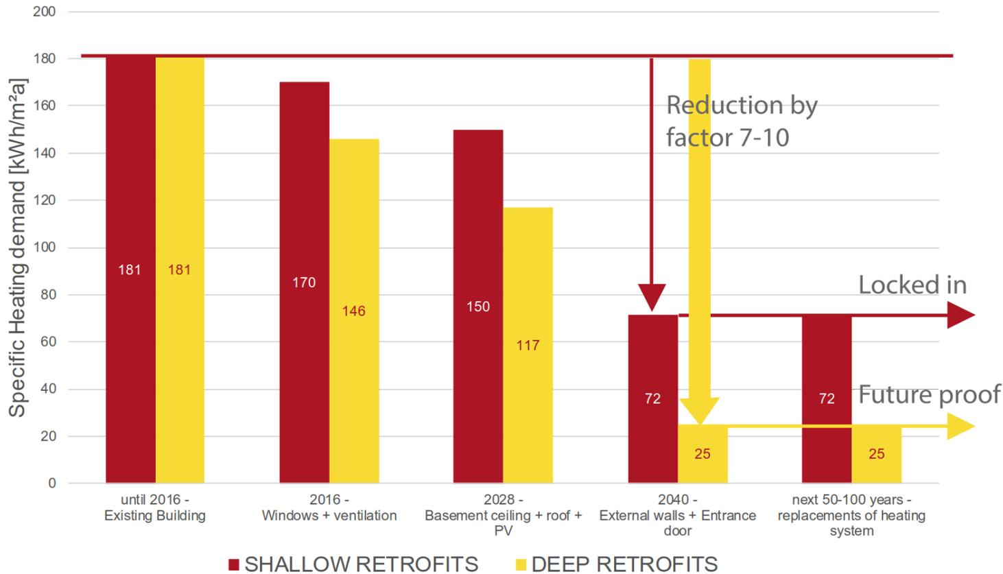
The graph shows the heating demand per m<sup>2</sup> of a house comparing shallow and deep energy retrofit measures following various retrofit steps over years. In the end, the house with the shallow measures applied has a heating demand 3 times as high as that of the deep retrofit measures.
